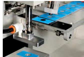
**Die Cutting:** This process cuts the custom design through the entire material. For example, when die cutting plastic with adhesive backing, the die cuts through the plastic face, adhesive, and backing material layers. The die cut design is fully separated from the stock material.
